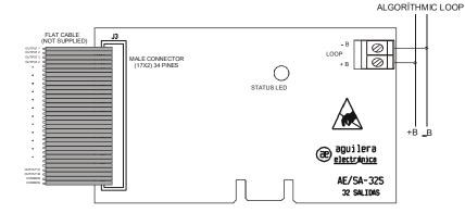
The AE/SA-32S module has a flat male ribbon connector with 17X2 pins for connection of the outputs. Pins number 33 and 34 are useful to do a global output test if you connect them to negative.
