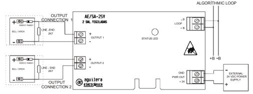
This module requires an auxiliary power supply of 24 Vdc for output actuation.
